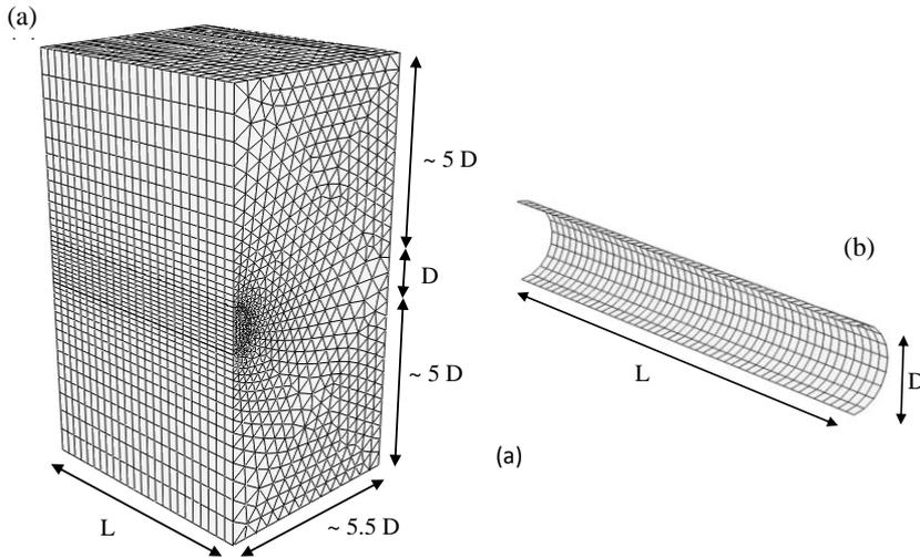
Fig. 1 (a) Adopted 3D FE mesh; (b) Detail of lining discretization.
