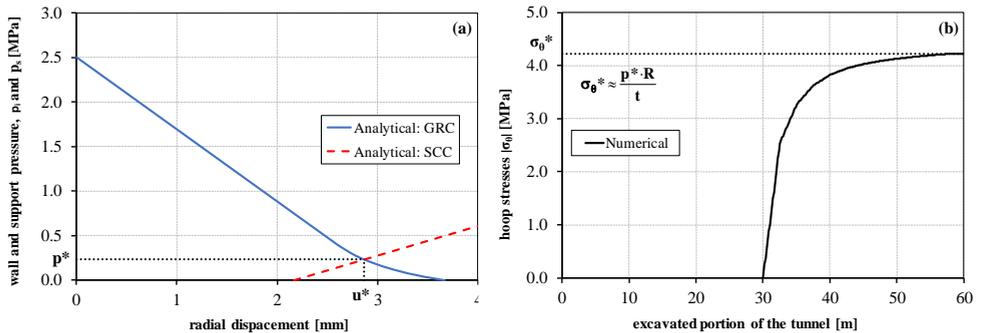
Fig. 2 (a) Analytical [9] representation of the Ground Reaction Curve (GRC) and Support Characteristic Curve (SCC), (b) Numerical hoop stresses in concrete lining.
