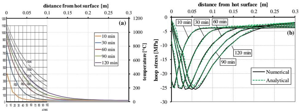
Fig. 3 (a) Temperature distribution across concrete lining thickness: comparison between numerical and EC2 [18] temperature profiles for concrete slabs; (b) Hoop stress distribution across concrete lining thickness: comparison between numerical and analytical [23] results.
