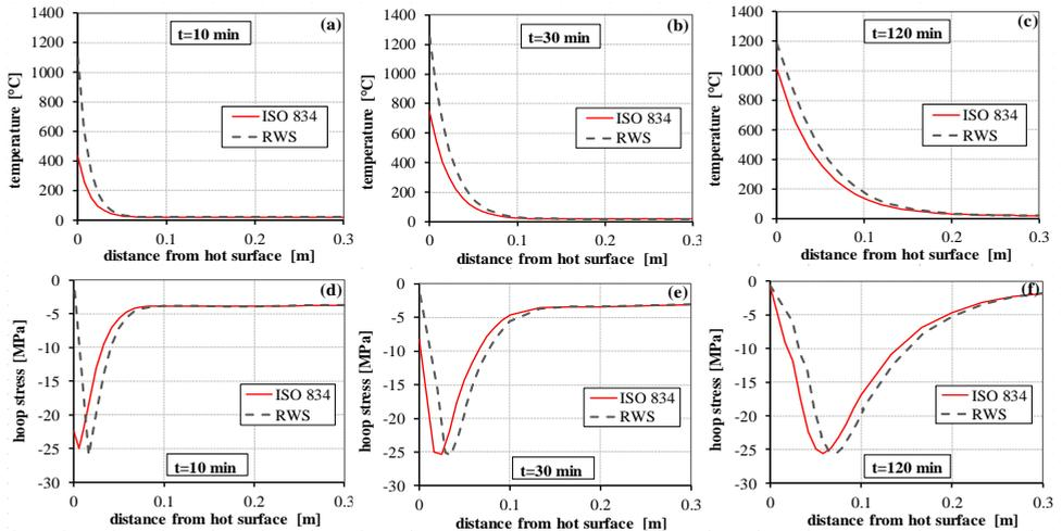
Fig. 4 (a), (b), (c) Temperature distribution and (b), (d), (f) hoop stress across concrete lining thickness at different fire exposure, obtained from 3D numerical analyses considering the ISO 834 and the RWS fire curves.
