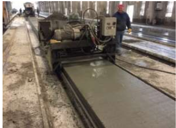
Figure 15. HC wall slabs, depth 150 mm, production on long casting beds with upper surface perfectly smoothed Pannelli alveolari parete, spessore 150 mm, liscati superiormente
